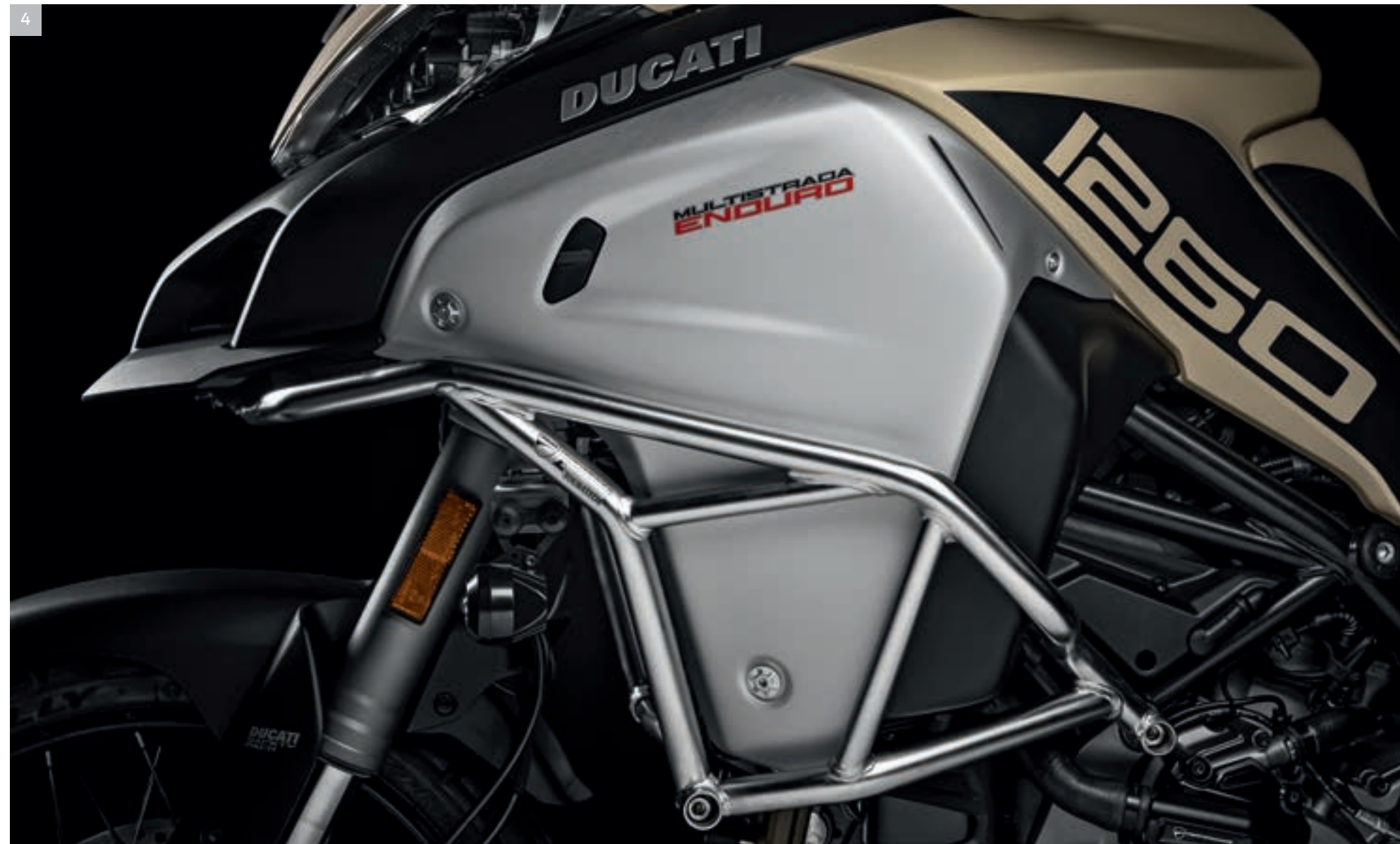
4 Side tank protectors in steel tubing
