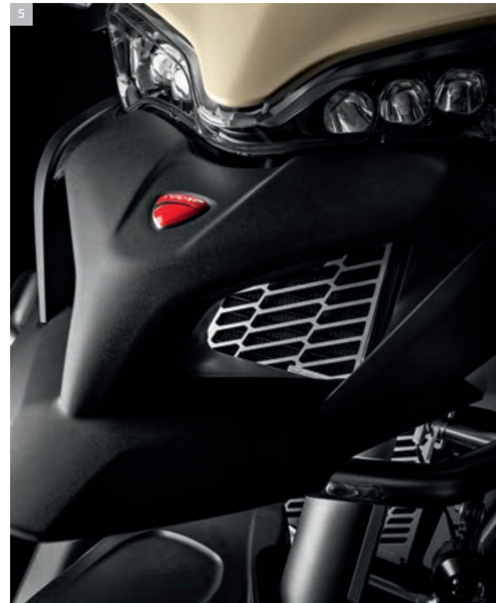
5 Protective mesh for oil cooler
